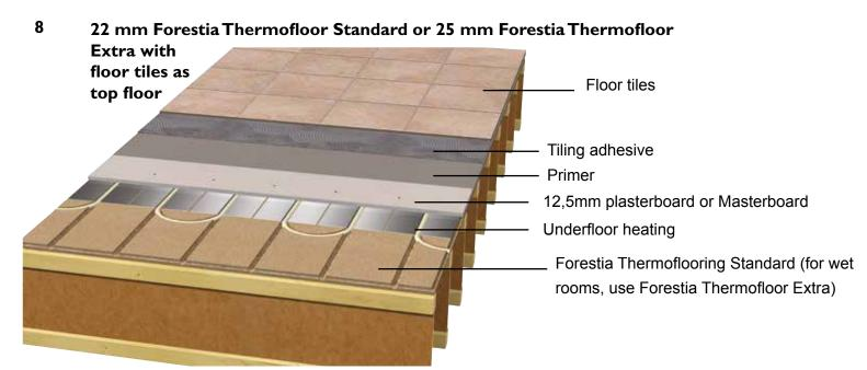
All floors with floor tiles must have joists at 300 mm centres. When installing in wet rooms, the membrane must be mounted between the primer and the tiling adhesive.
